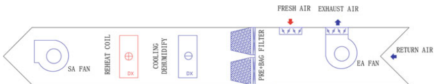
Fig. 7.5 Cooling and reheating coils
