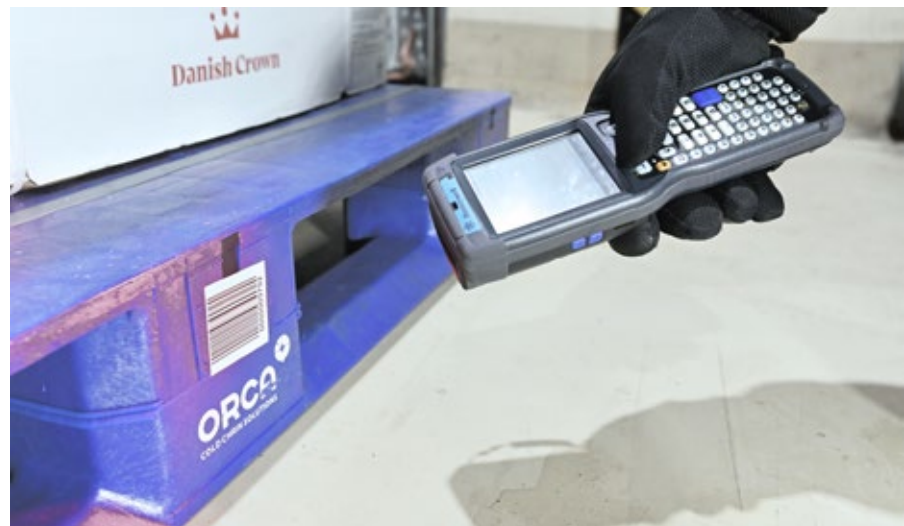
Tagging of pallets using QR codes for real-time monitoring.
