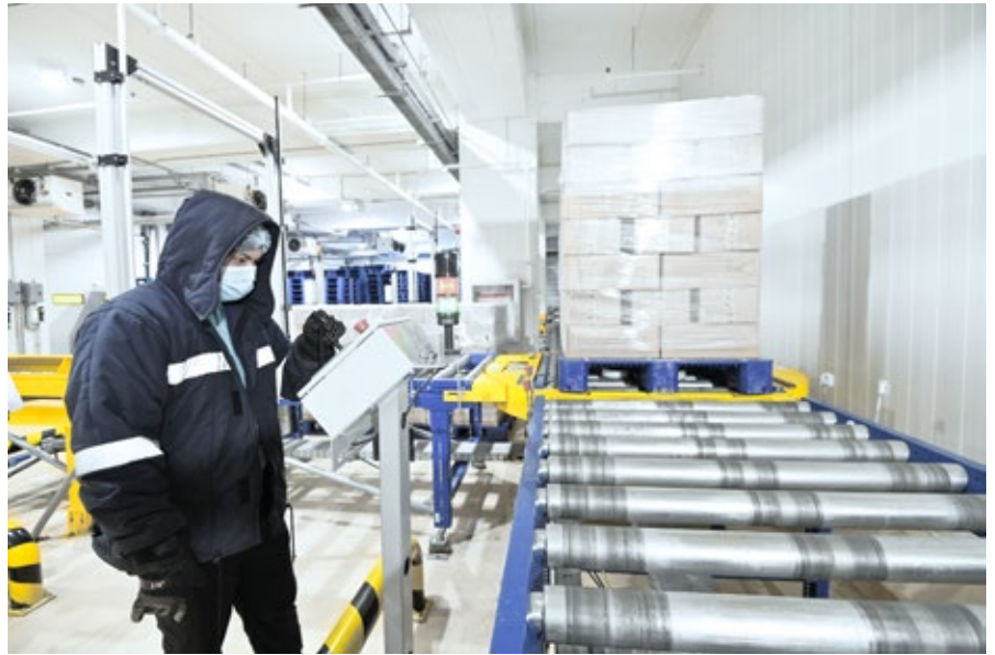
Pallets are transferred from a -18°C environment to the automated high-bay warehouse via conveyors.
