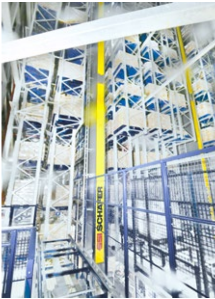
The four SSI Exyz storage-retrieval machines operate simultaneously and are unaffected by the sub-zero temperatures.
